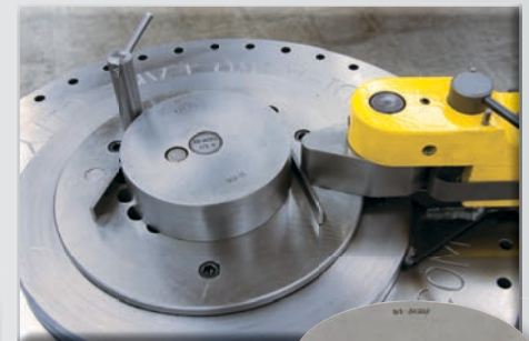
Radius Collar - Style B Used with standard Locking Pin; for forming solid material.
