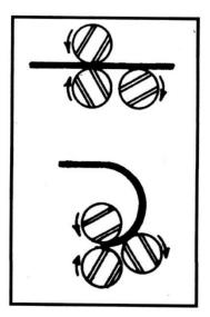
AFTER HALF CIRCLE-has been formed, reinsert the formed end of the material into the roller (as illustrated) and turn operating handle in a clockwise direction to form a complete circle.
